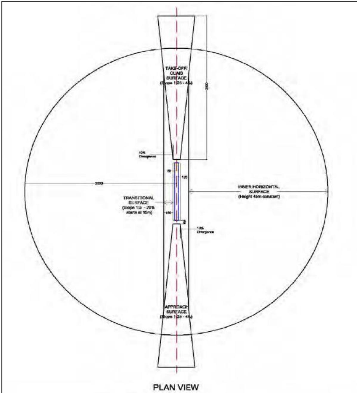
Figure G-1(A) Water Aerodrome Obstacle Limitation Surface
