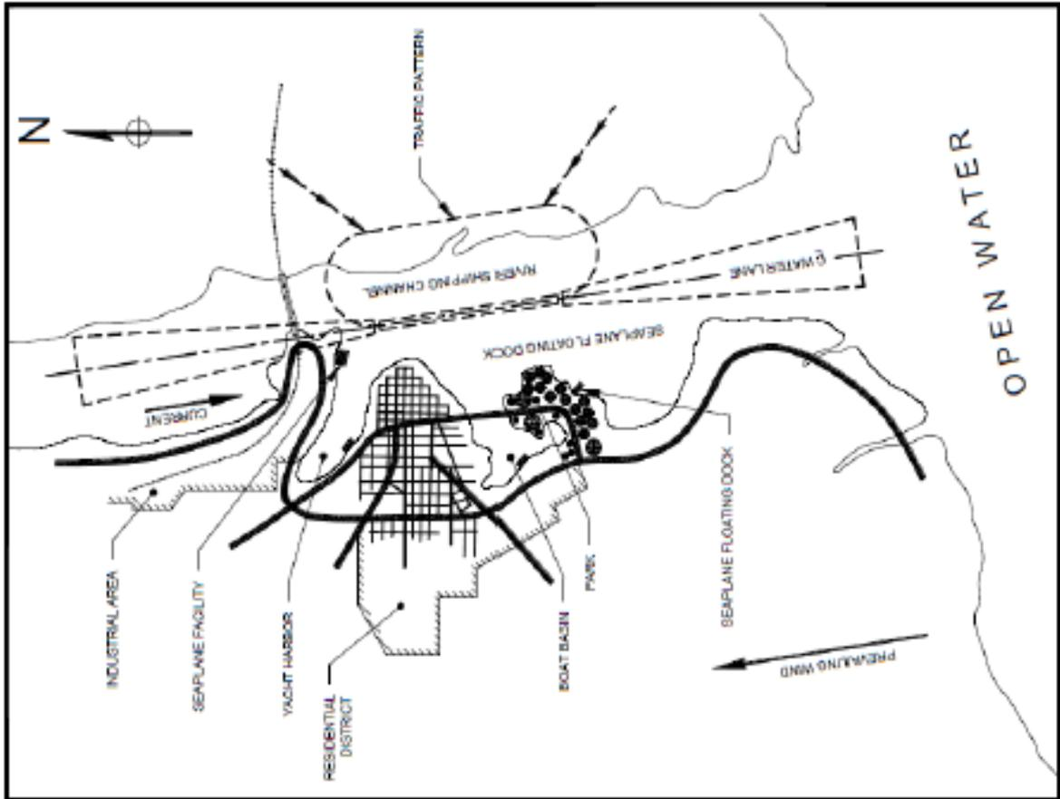
(Fig Appendix: A3-1 Example of location of water aerodrome and water runway
