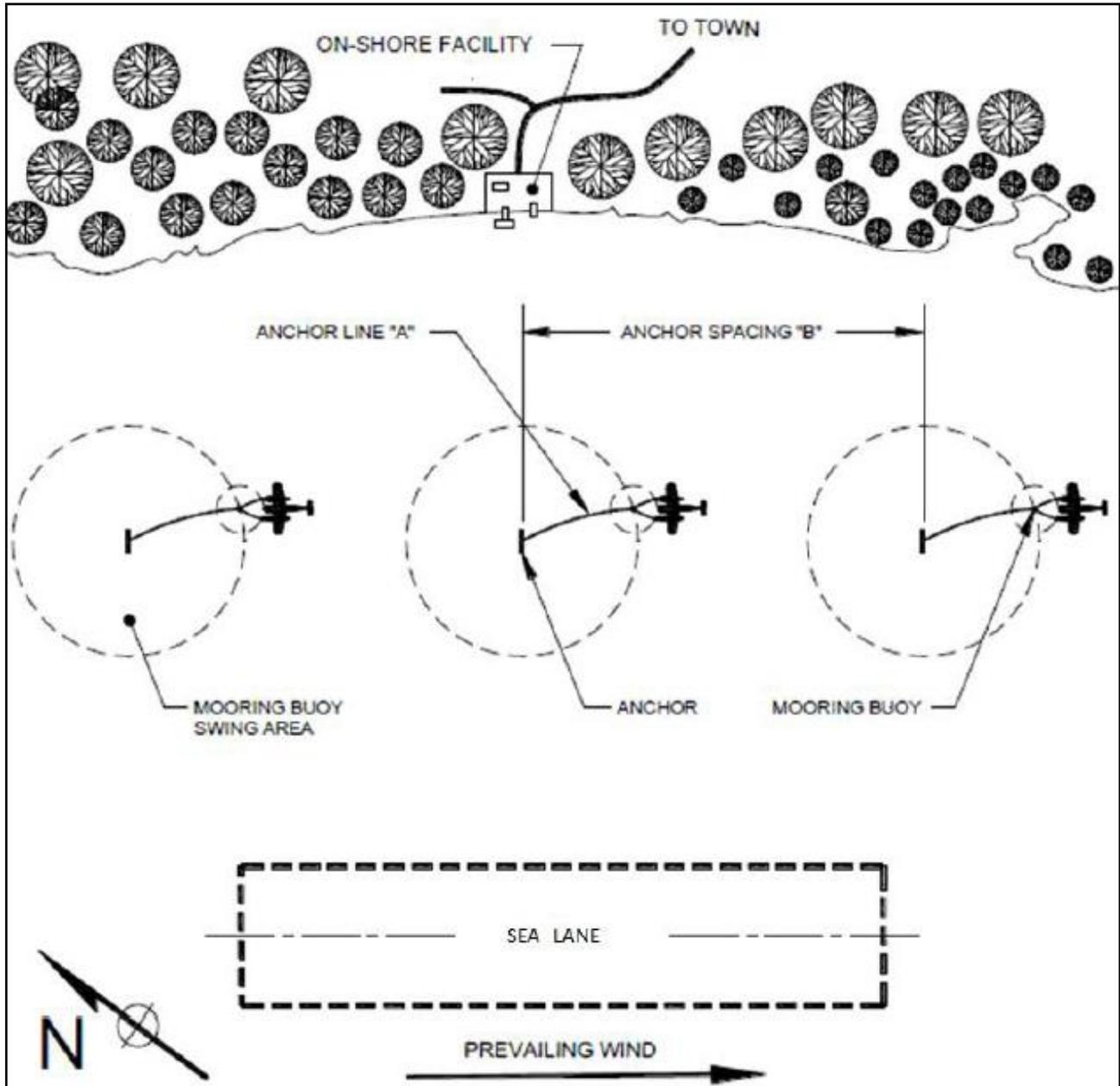
**Figure F-3. Illustration of an anchorage area with permanent mooring buoys swing areas**
