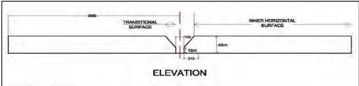
**Figure G-1(B) Water Aerodrome Obstacle Limitation Surface**
